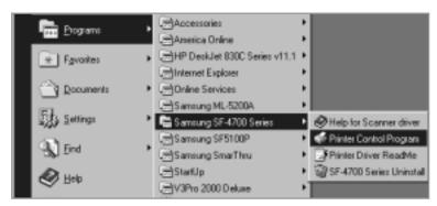
3. Samsung SF-4700 Series Control Program on LPT1 dialogue box appears. Select the **Cartridges** tab.
